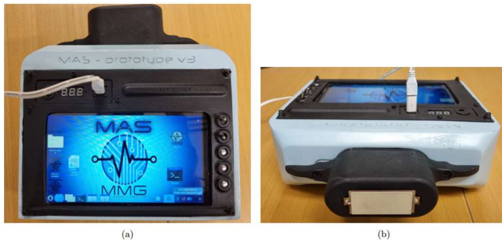
Figure 1: (a) The MAS device, (b) The top perspective of the MAS device showing where the sensor will be connected.
